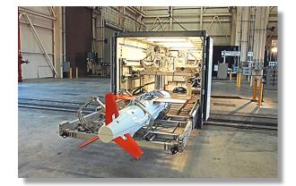
The LCS Mine Counter-Measure module is comprised of five different Mission Modules that consist of low-weight, high-strength steel containers that store, restrain, and house high precision electronic sensors and equipment used in the various ship missions.
